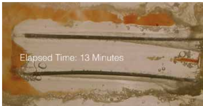
Figure 12: The isthmus block result after just 13 minutes when the vacuum was reversed to prevent cannula blockage and found that the constant vacuum-drawn outflow through the end of the cannula radically increased dissolution speed
