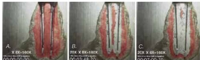
Figures 17A-17C: Isthmus research blocks showing the isthmus replica dissolved in 7 minutes with higher NaOCl concentrations, temperatures, and continuous agitation from aeration bubbles
